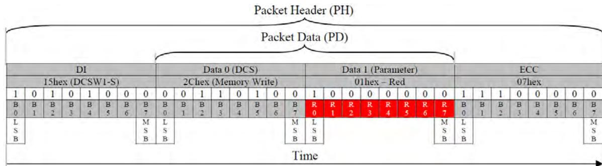
Figure 92: Red Sub-pixel Write (DCSW1-S) – Example 4
