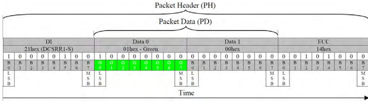
Figure 96: Green Sub-pixel Response (DCSRR1-S) – Example 3
