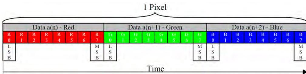
**Figure 88: One Pixel Bit and Color Write Orders**
