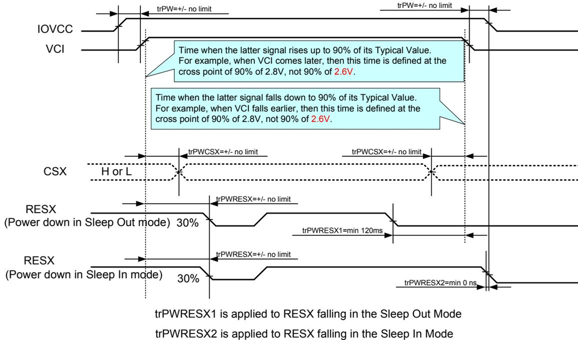
**Note:** Unless otherwise specified, timings herein show the cross point at 50% of the signal power level.
