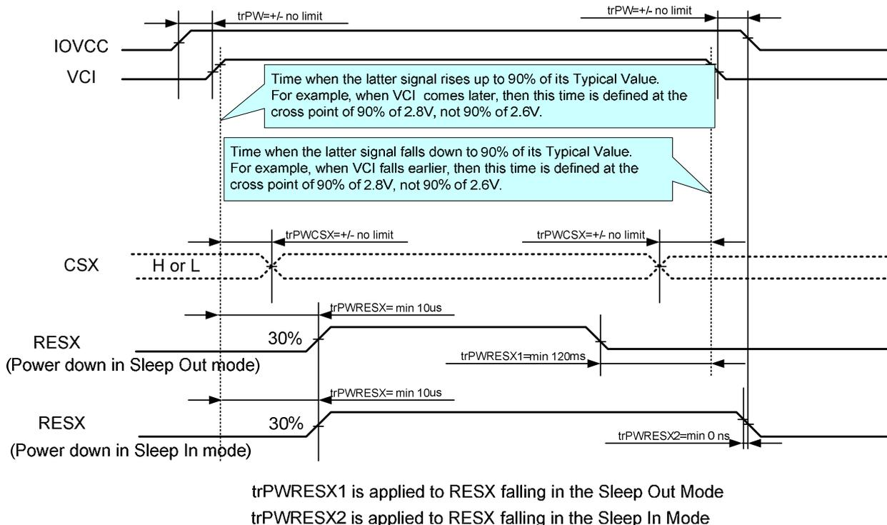
**Note:** Unless otherwise specified, timings herein show the cross point at 50% of the signal power level.
