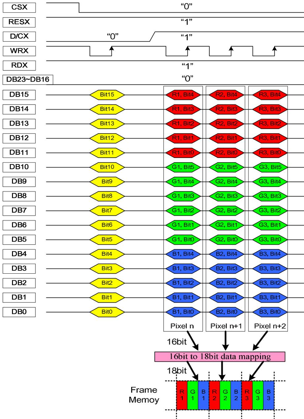
**Figure 115: 16-bit Data Bus for 16-bit/pixel (RGB 5-6-5 Bits Input), 65K-color**
