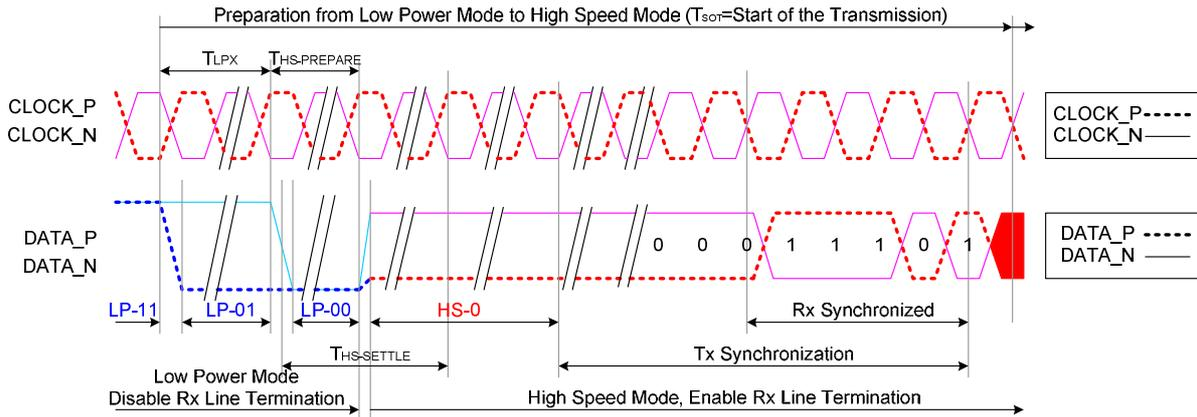
**Figure 37: Entering High-Speed Data Transmission (T<sub>SOT</sub> of HSDT)**
