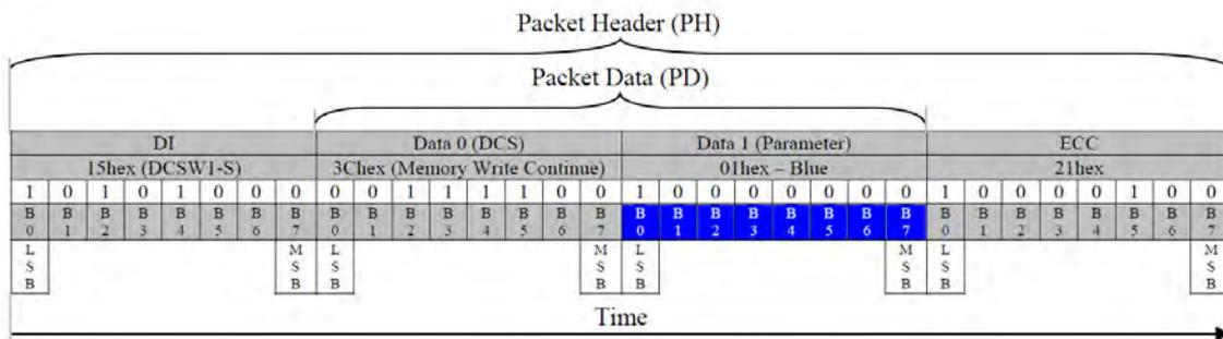
**Figure 90: Blue Sub-pixel Write (DCSW1-S) – Example 2**
