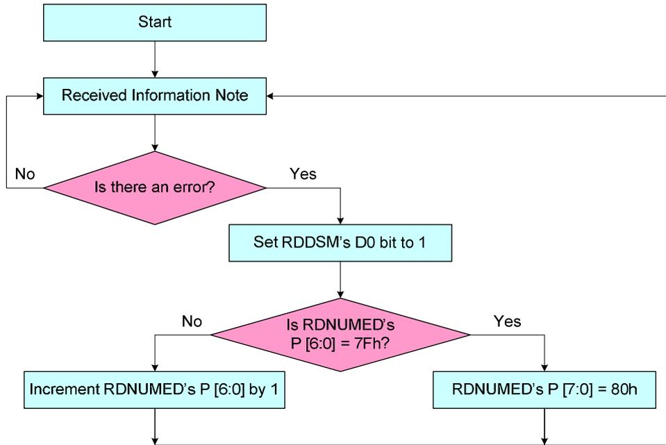
**Figure 80: Flow Chart for Errors on DSI**
