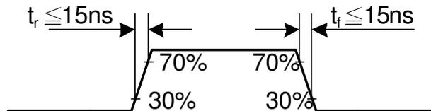
**18.3.5 Parallel 18/16/6-bit RGB Interface Timing Characteristics**
