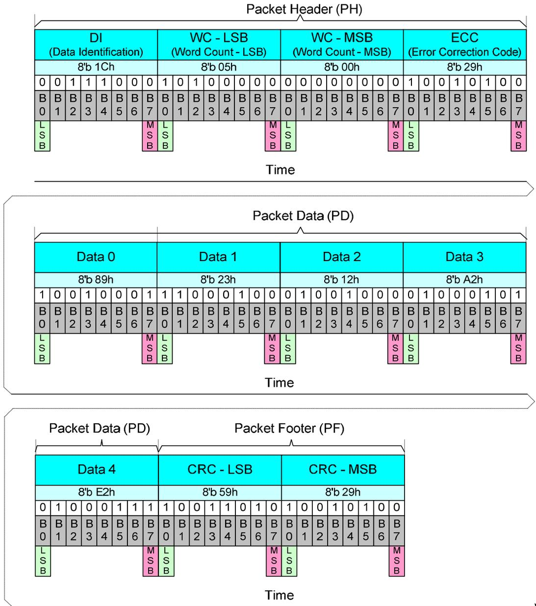
Figure 81: DCS Read Long Response (DCSRR-L) – Example
