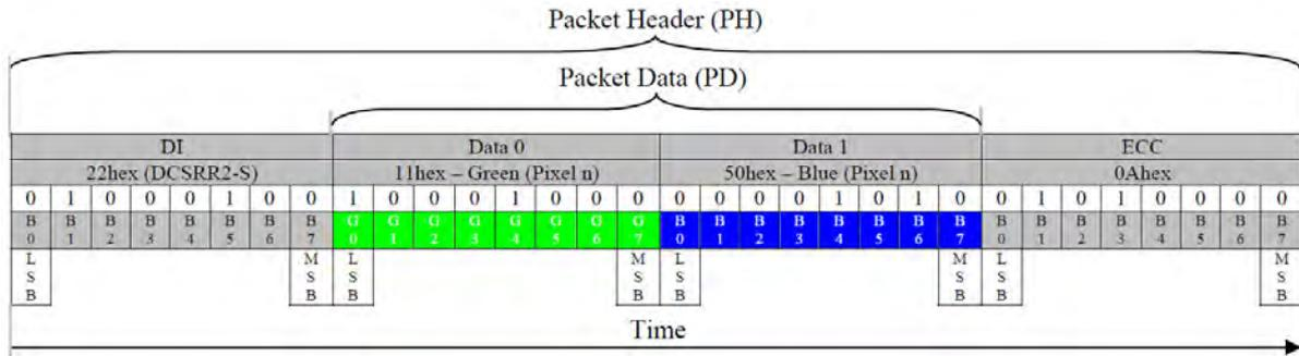
**Figure 99: Green and Blue Sub-pixels Response (DCSRR2-S) – Example 6**
