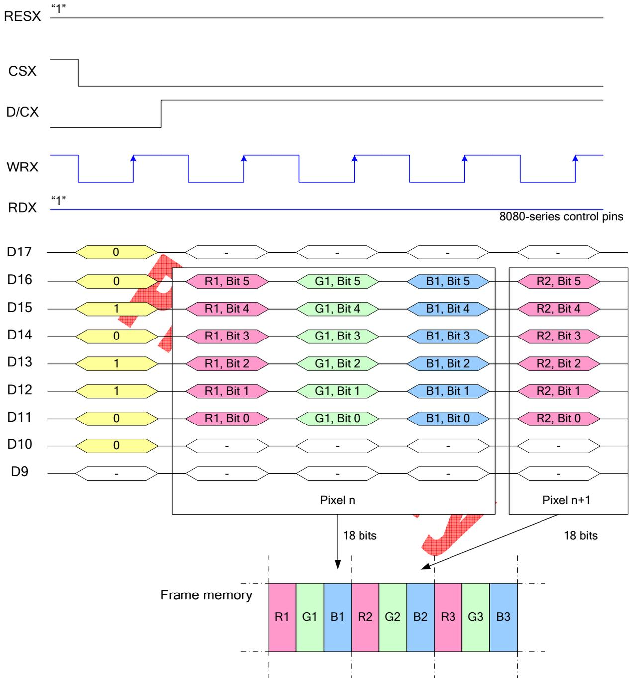
Note 1: The data order is as follows, MSB=D16, LSB=D11 and picture data is MSB=Bit 5, LSB=Bit 0 for Red, Green and Blue data.
