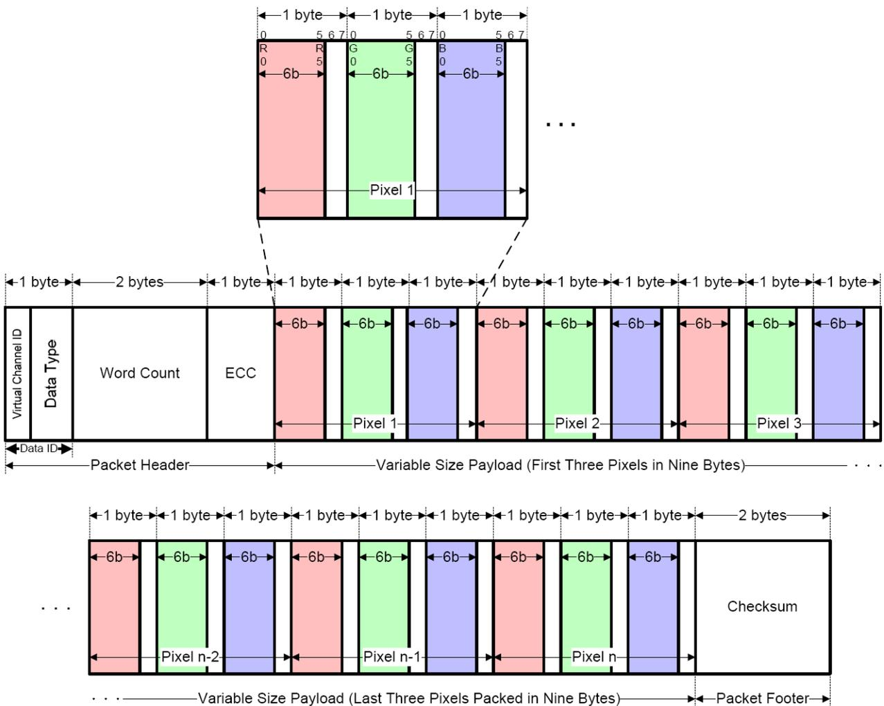
**Figure 127: 18-bit per Pixel, Data Type = 10 1110 (2Eh)**
