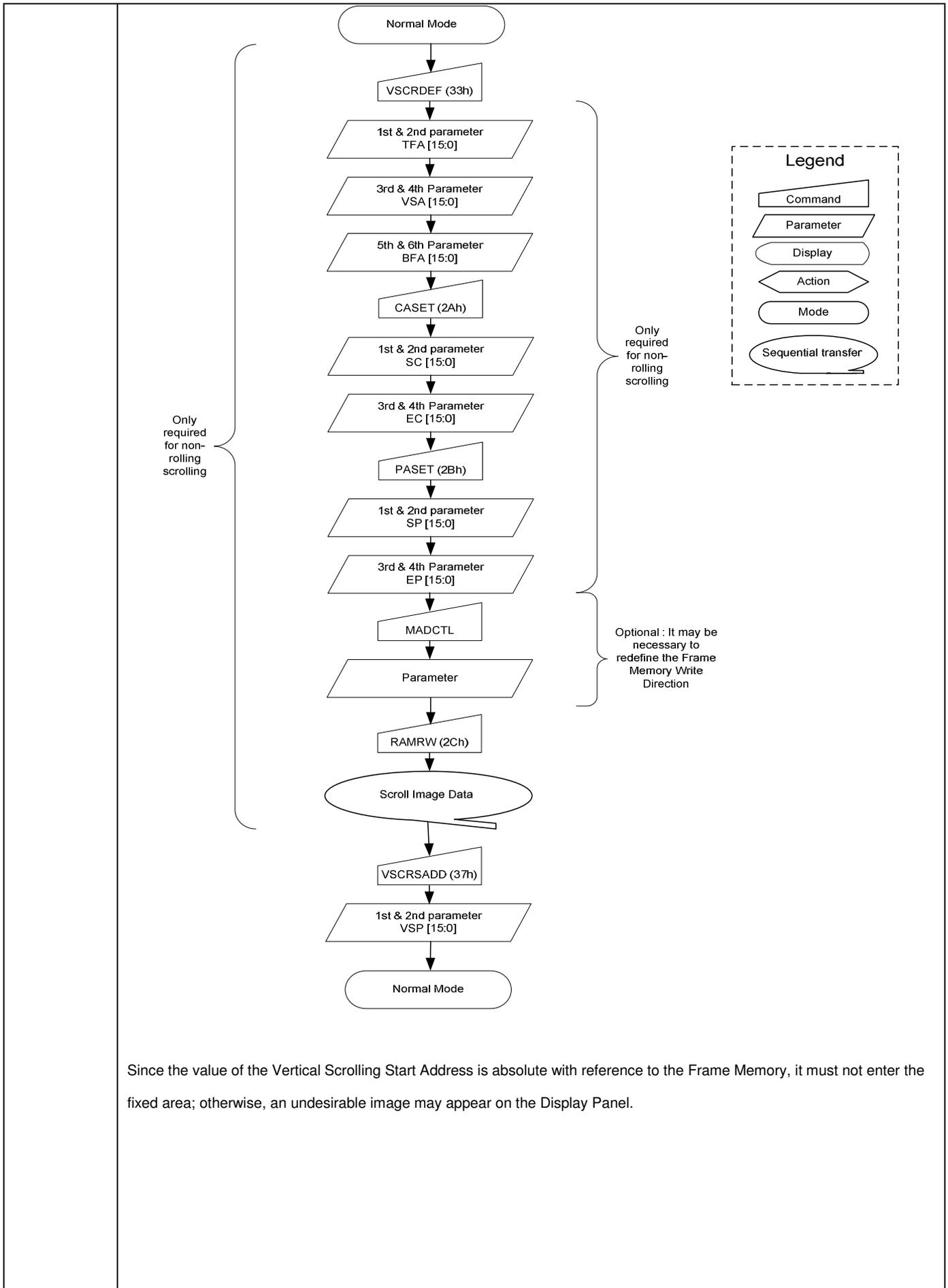
Since the value of the Vertical Scrolling Start Address is absolute with reference to the Frame Memory, it must not enter the fixed area; otherwise, an undesirable image may appear on the Display Panel.
