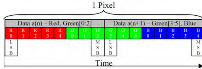
**Figure 84: One Pixel Bit and Write Color Orders**
