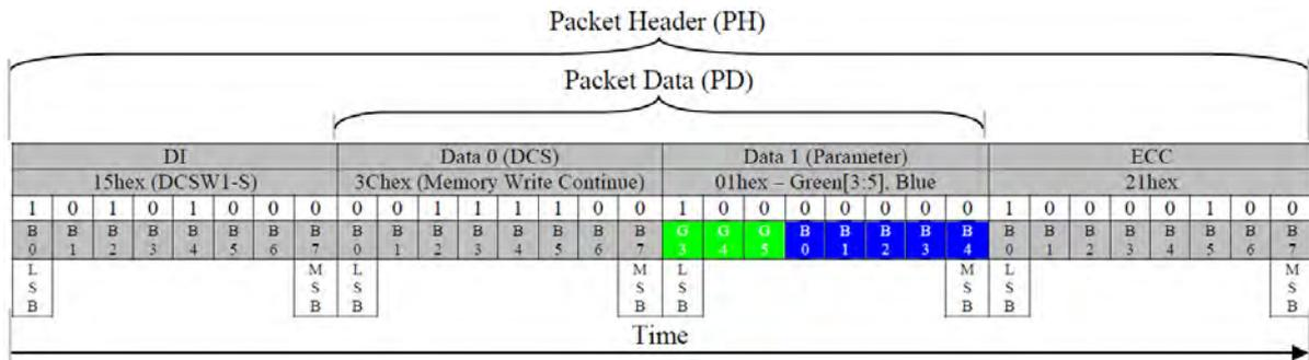
**Figure 87: Green [3:5]/Blue Sub-pixel Write (DCSW1-S) – Example 3**
