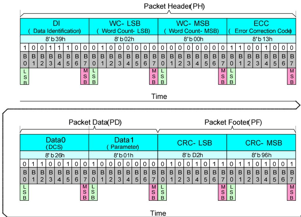
**Figure 69: Display Command Set Write Long (DCSW-L) with DCS and 1 Parameter – Example**
