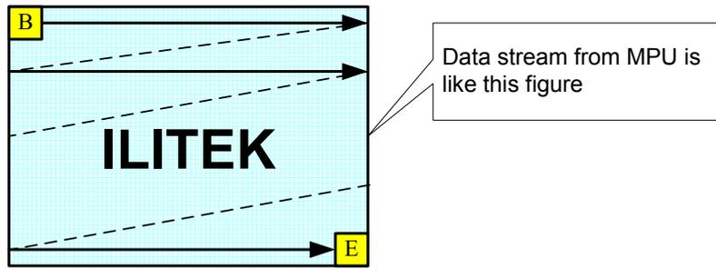
The data is written in the order illustrated above. The Counter, indicating where in the physical memory the data is to be written, is controlled by the Memory Data Access Control Command, Bits D7, D6, and D5, as described below.
