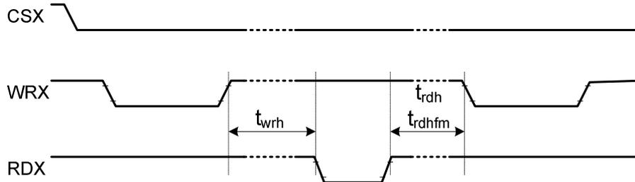
**17.4.2. DBI Type C Option 1 (3-Line SPI System) Timing Characteristics**
