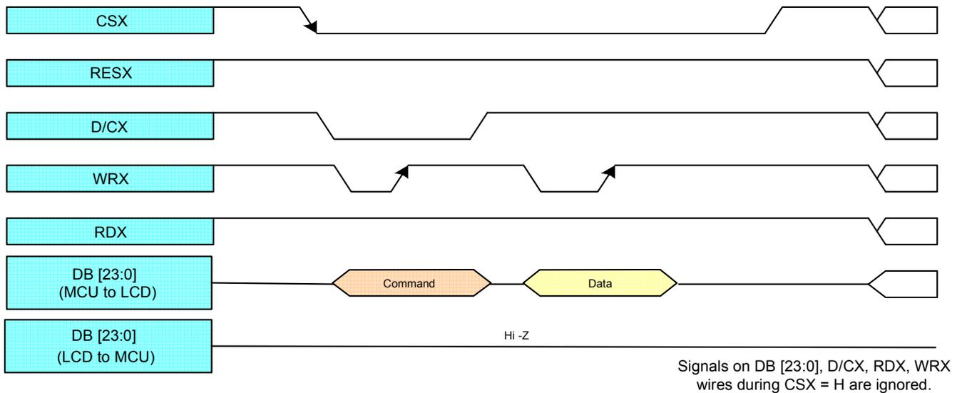
**Figure 2: DBI Type B Write Cycle Sequence**
