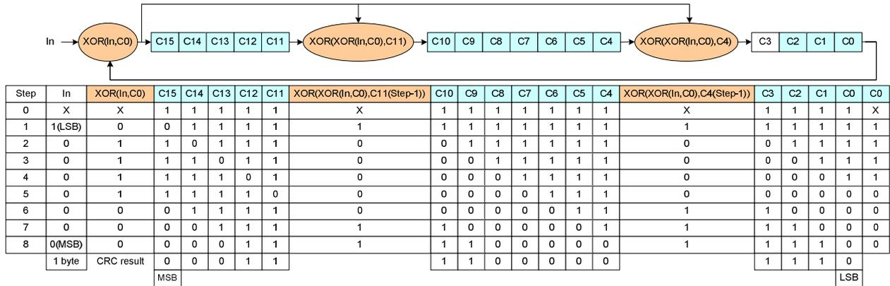
**Figure 63: CRC Calculation – Packet Data (PD) is 01h**
