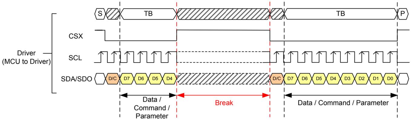
**Figure 11: Data Transfer Break and Recovery**
