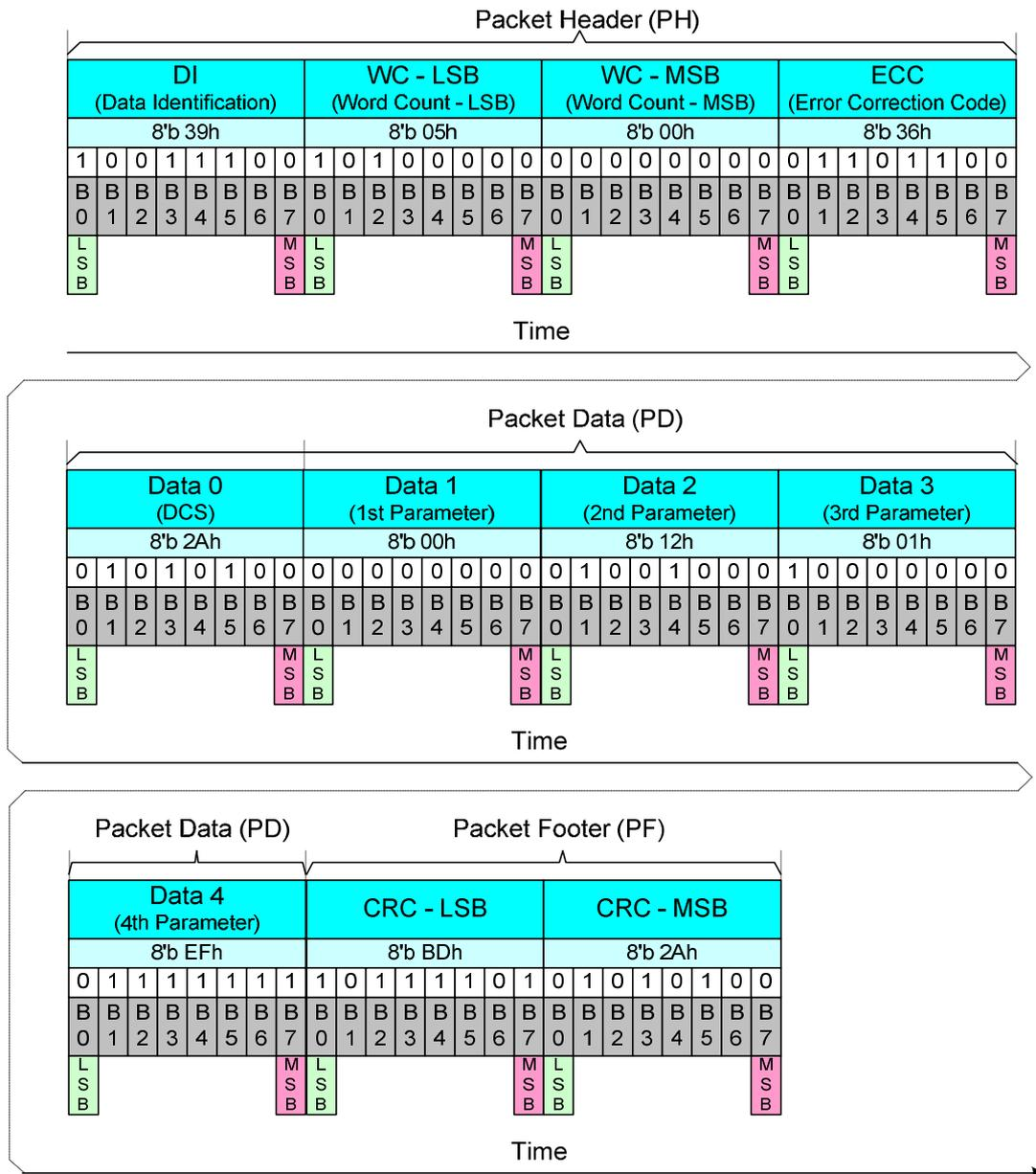
Figure 70: Display Command Set Write Long with DCS and 4 Parameters – Example
