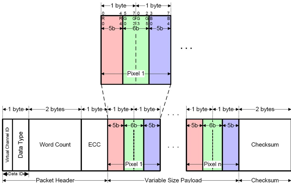
Figure 125: 16-bit per Pixel, Data Type 00 1110 (0Eh)
