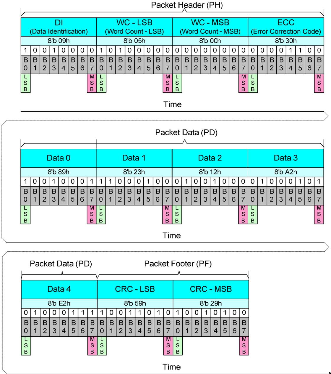
Figure 73: Null Packet, No Data (NP-L) – Example
