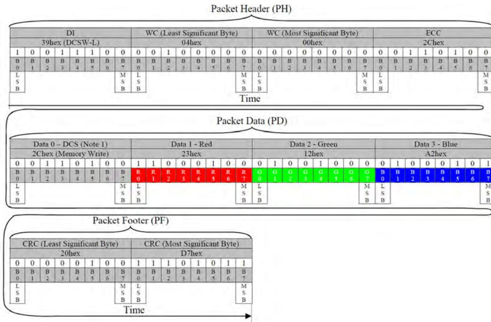
**Figure 89: One Pixel Write (DCSW-L) – Example 1**
