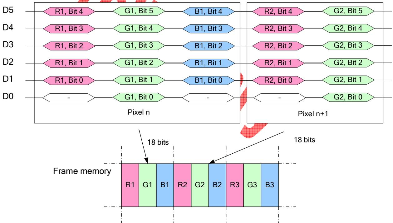
Write data for 6-bit/pixel (RGB 6-6-6-bit input), 262K-Colors
