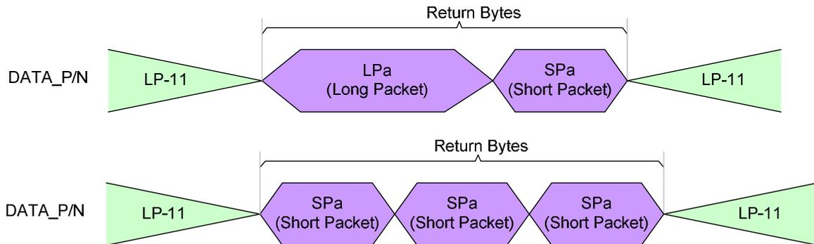
**Figure 77: Return Bytes in Multiple Packets – Now Allowed**
