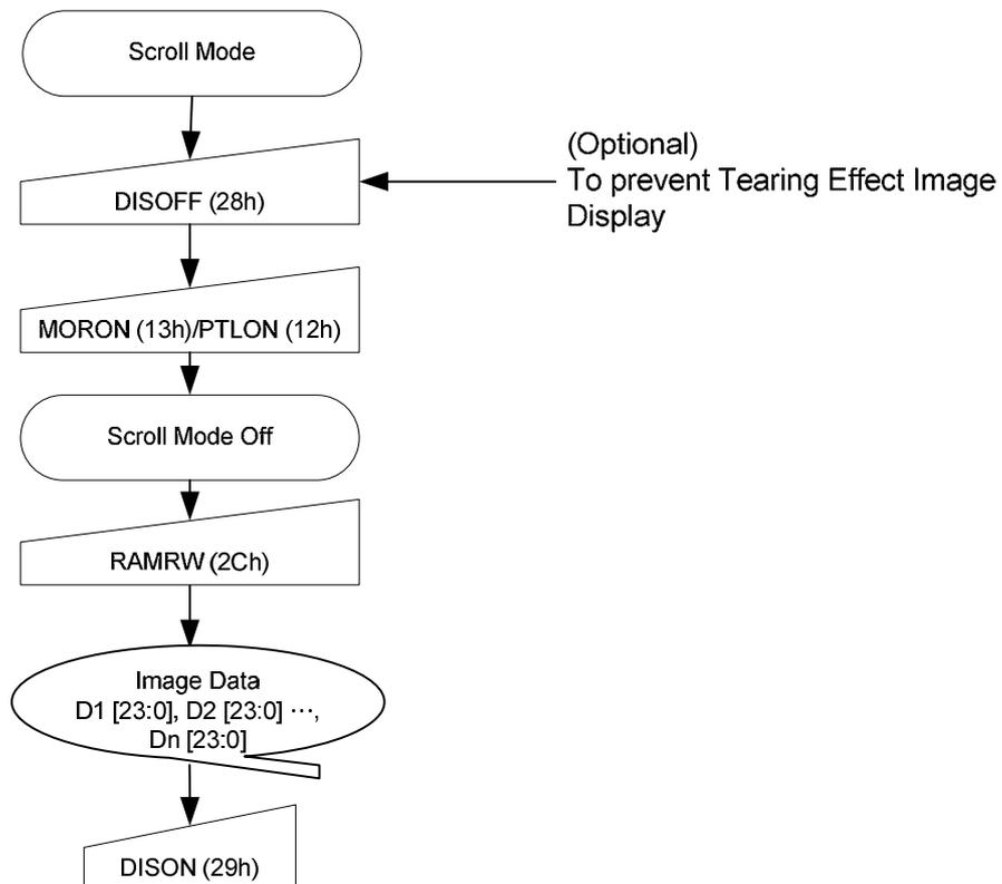
**Note:** To exit the Scroll Mode, both Normal Display Mode On (13h) and Partial Mode On (12h) commands can be used.
