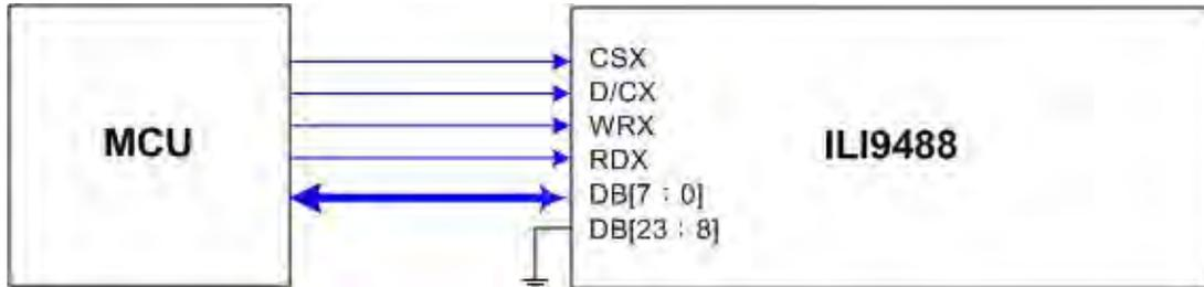
Figure 109: 8-bit Parallel MCU Interface
