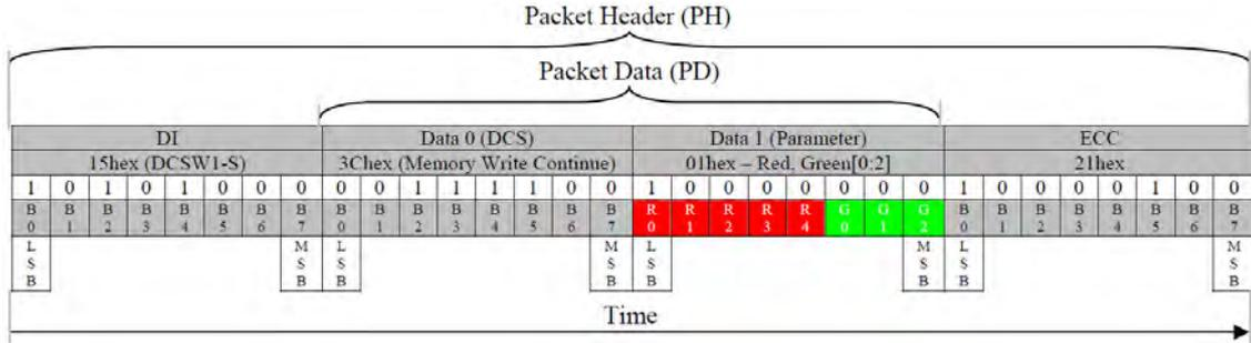
**Figure 86: Red/Green [0:2] Sub-pixel Write (DCSW1-S) – Example 2**
