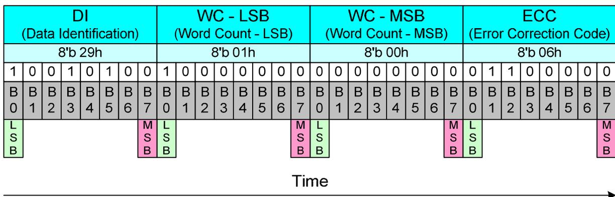
**Figure 44: Bit Order of Bytes in Packets**
