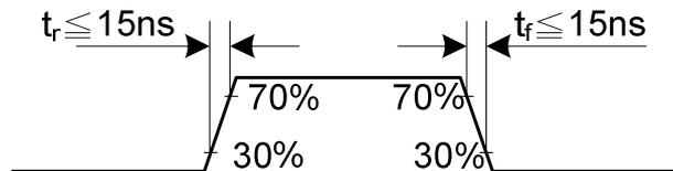
**17.4.3. DBI Type C Option 3 (4-Line SPI System) Timing Characteristics**
