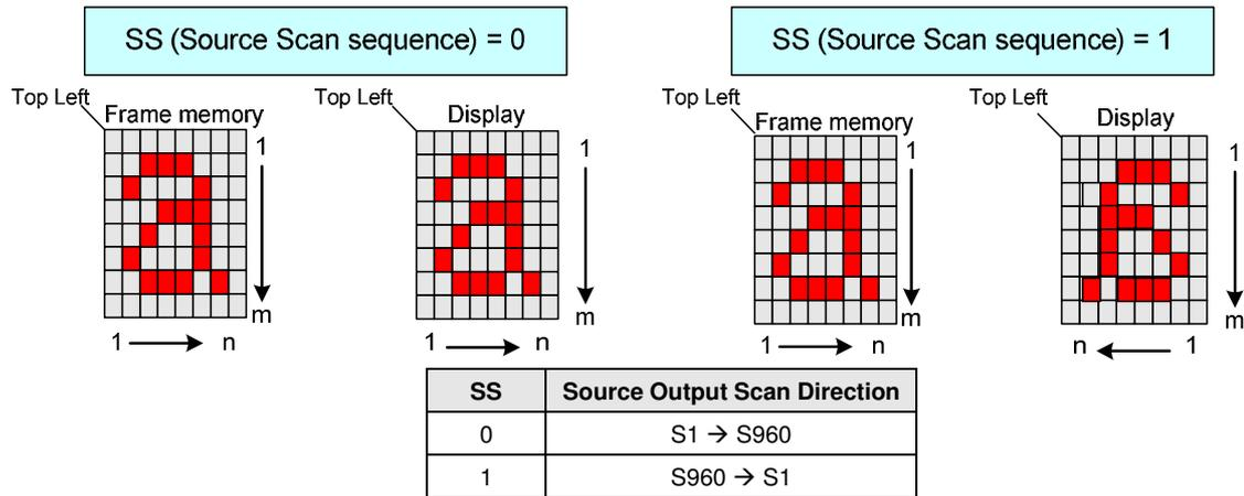
In addition to the shift direction, the settings for both SS and BGR bits are required to change the assignment of R, G, B dots to the source driver pins.
