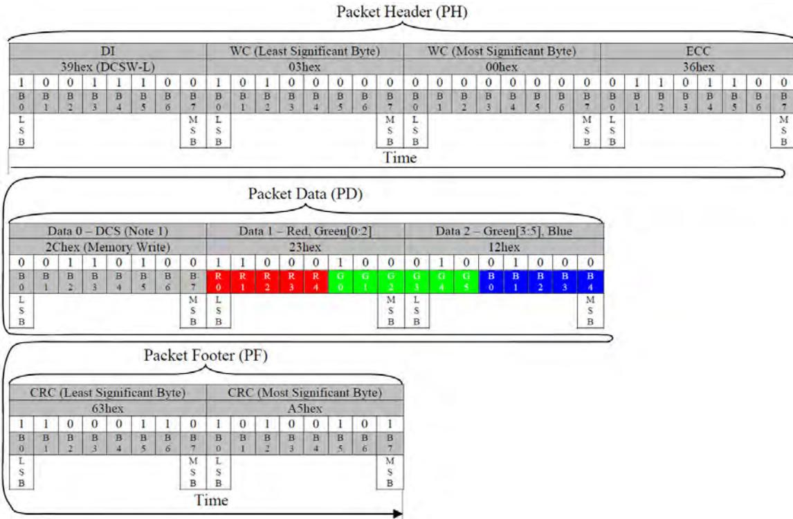
**Figure 85: One Pixel Write (DCSW-L) – Example 1**
