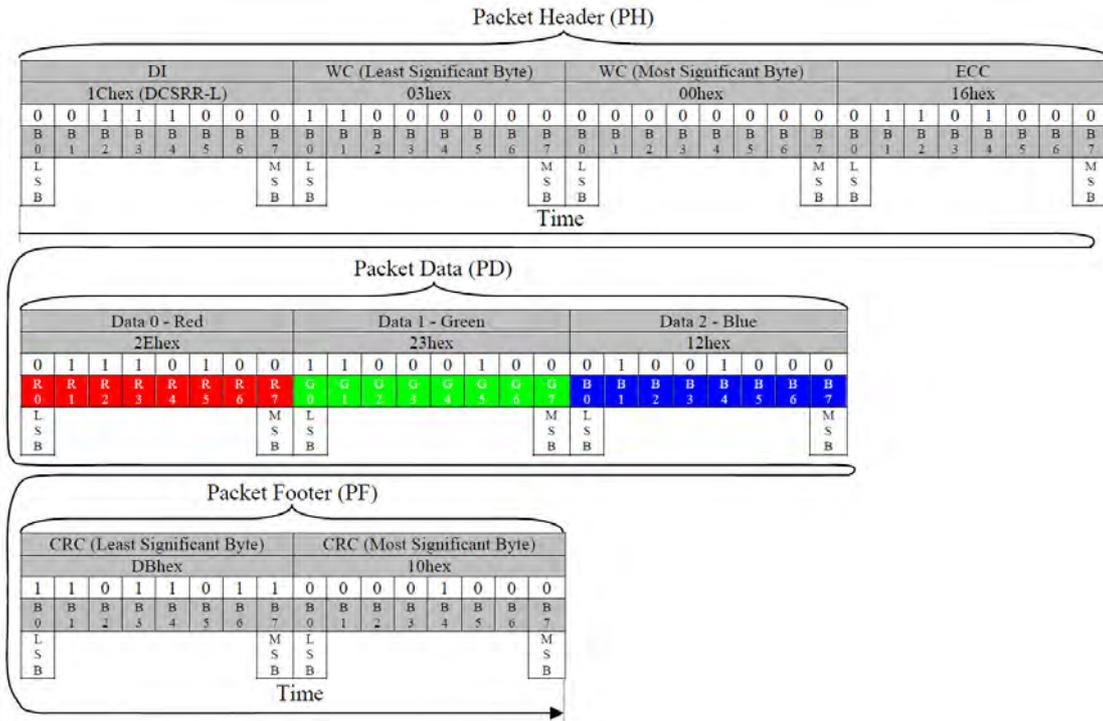
**Figure 94: One Pixel Read Response (DCSRR-L) – Example 1**
