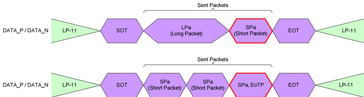
**Figure 75: End of Transmission Packet (EoTP) – Examples**
