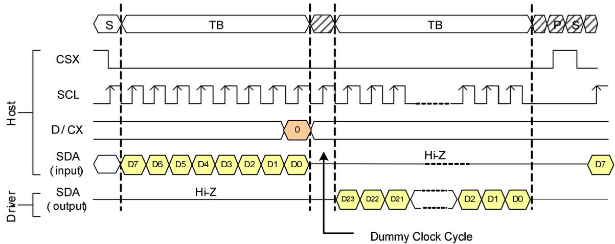
4-line Serial Protocol (for RDDST command: 32-bit read)
