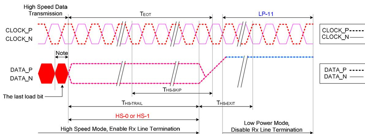
**Figure 38: Leaving High-Speed Data Transmission**
