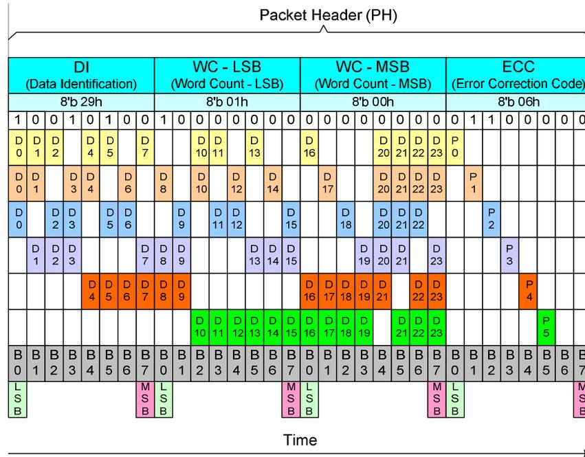
**Figure 59: XOR Function on a Long Packet**
