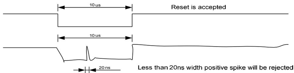
**Figure 137: Positive Noise Pulse during Reset Low**
