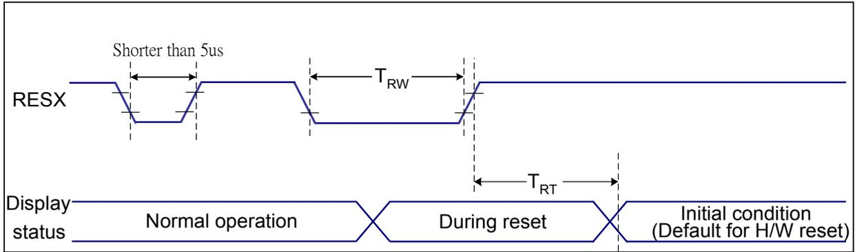
Figure 7 Reset Timing
