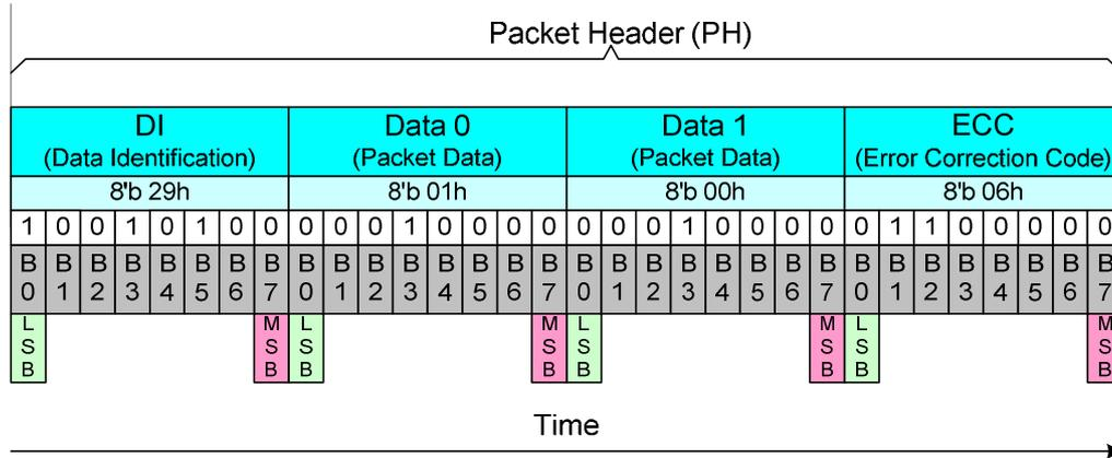
**Figure 47: Packet Header (PH) of Long Packet**
