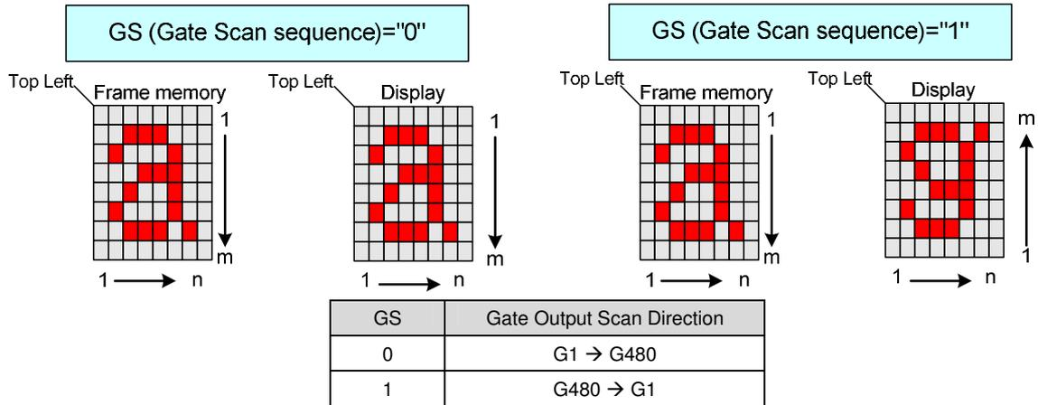
**SM:** Set the gate driver pin arrangement in combination with the GS bit (RB6h) to select the optimal scan mode for the module.
