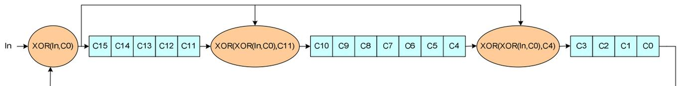
**Figure 62: 16-bit Cyclic Redundancy Check (CRC) Calculation**
