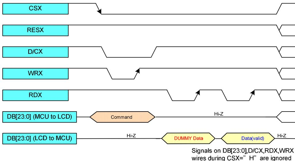
**Figure 4: DBI Type B Read Cycle Sequence**
