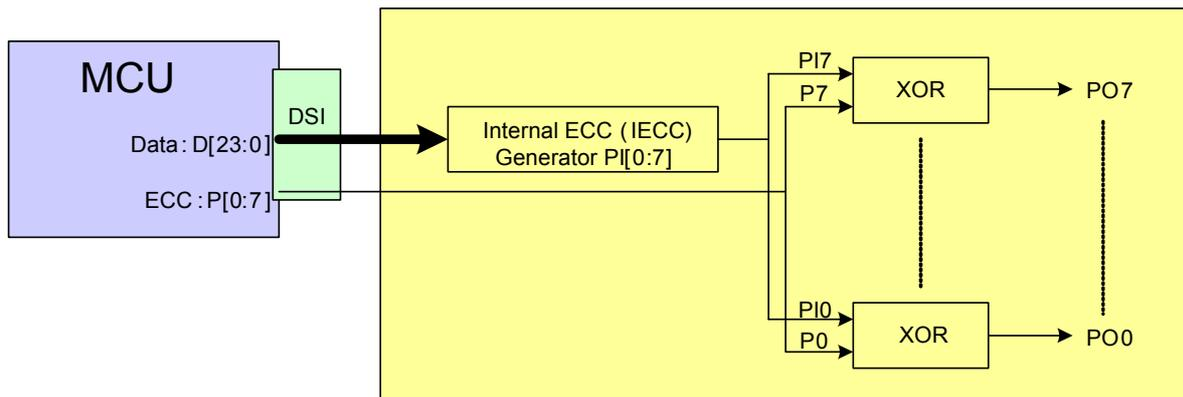
The sent data bits (D [23...0]) and ECC (P [7...0]) are received correctly, if the value of the PO [7...0] is 00h. The sent data bits (D [23...0]) and ECC (P [7...0]) are not received correctly, if the value of the PO [7...0] is not 00h.
