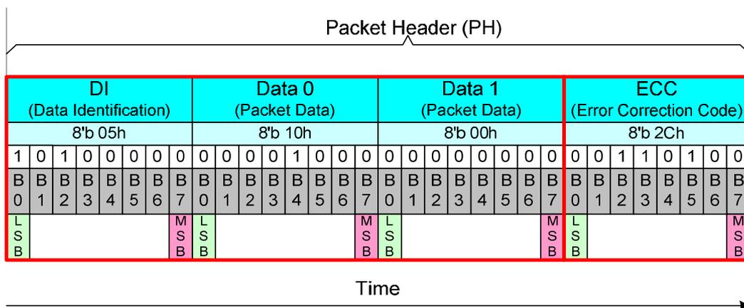
**Figure 56: D [23...0] and P [7...0] in a Short Packet**
