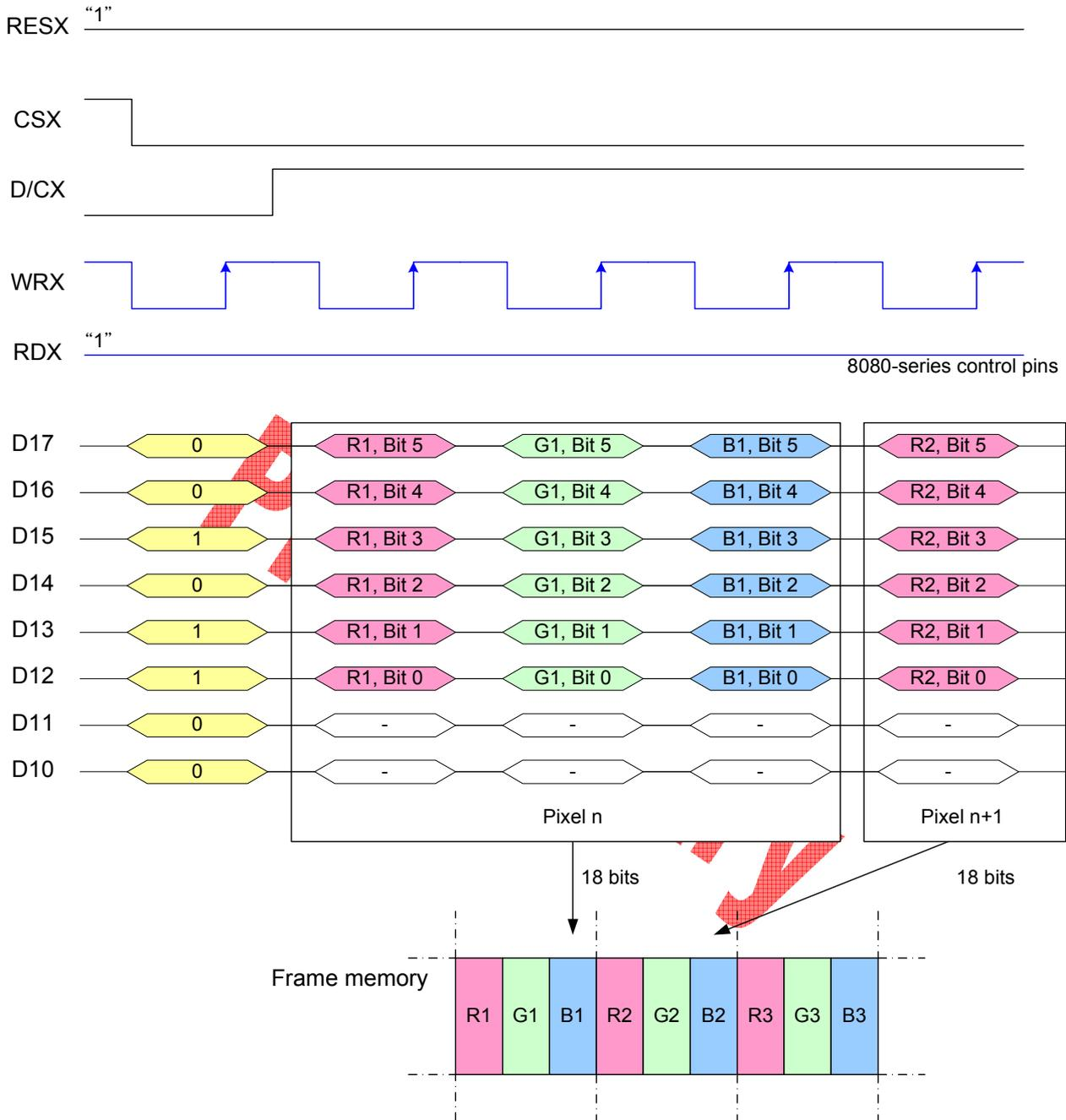
Note 1: The data order is as follows, MSB=D17, LSB=D10 and picture data is MSB=Bit 5, LSB=Bit 0 for Red, Green and Blue data.
