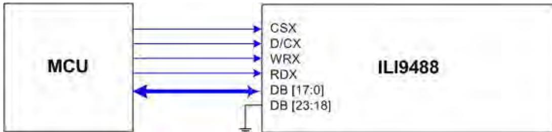
**Figure 117: 18-bit Parallel MCU Interface**
