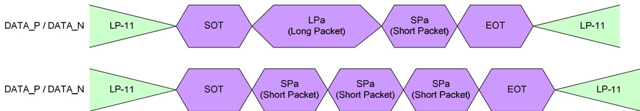
**Figure 40: Multiple Packets in High-Speed Data Transmission (Examples)**
