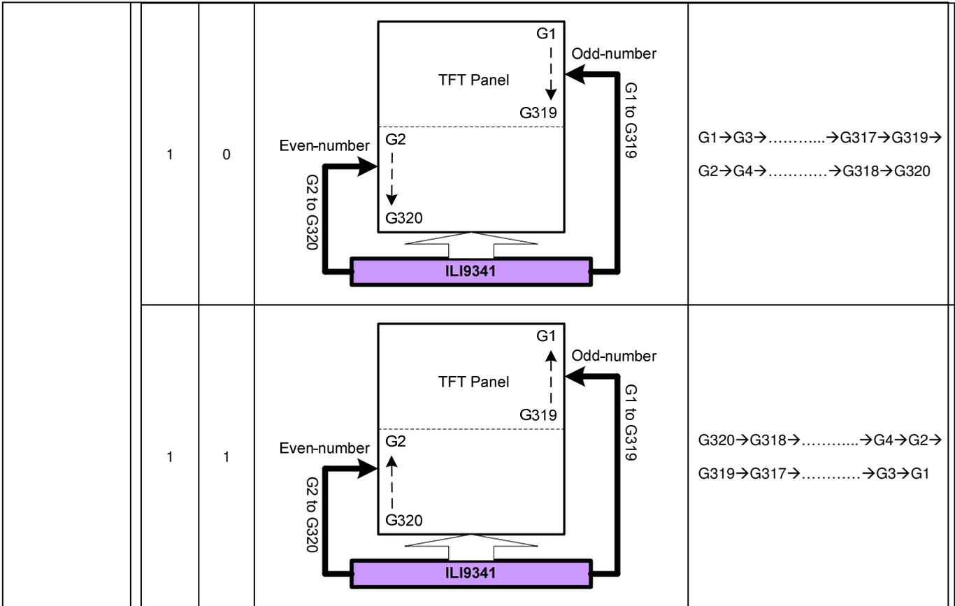
**NL [5:0]:** Sets the number of lines to drive the LCD at an interval of 8 lines. The GRAM address mapping is not affected by the number of lines set by NL [5:0]. The number of lines must be the same or more than the number of lines necessary for the size of the liquid crystal panel.
