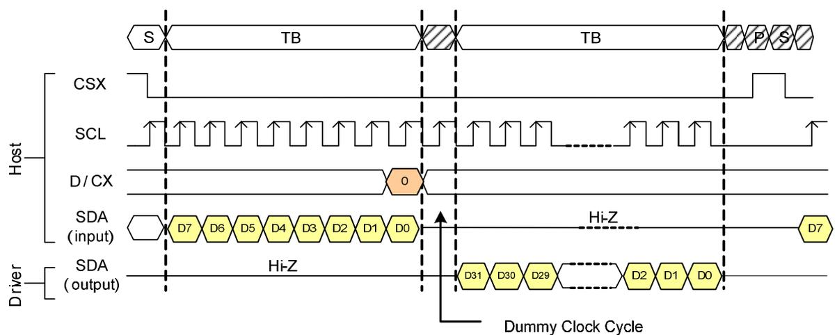
Figure 10: DBI Type C (Option 3) Read Cycle Sequence
