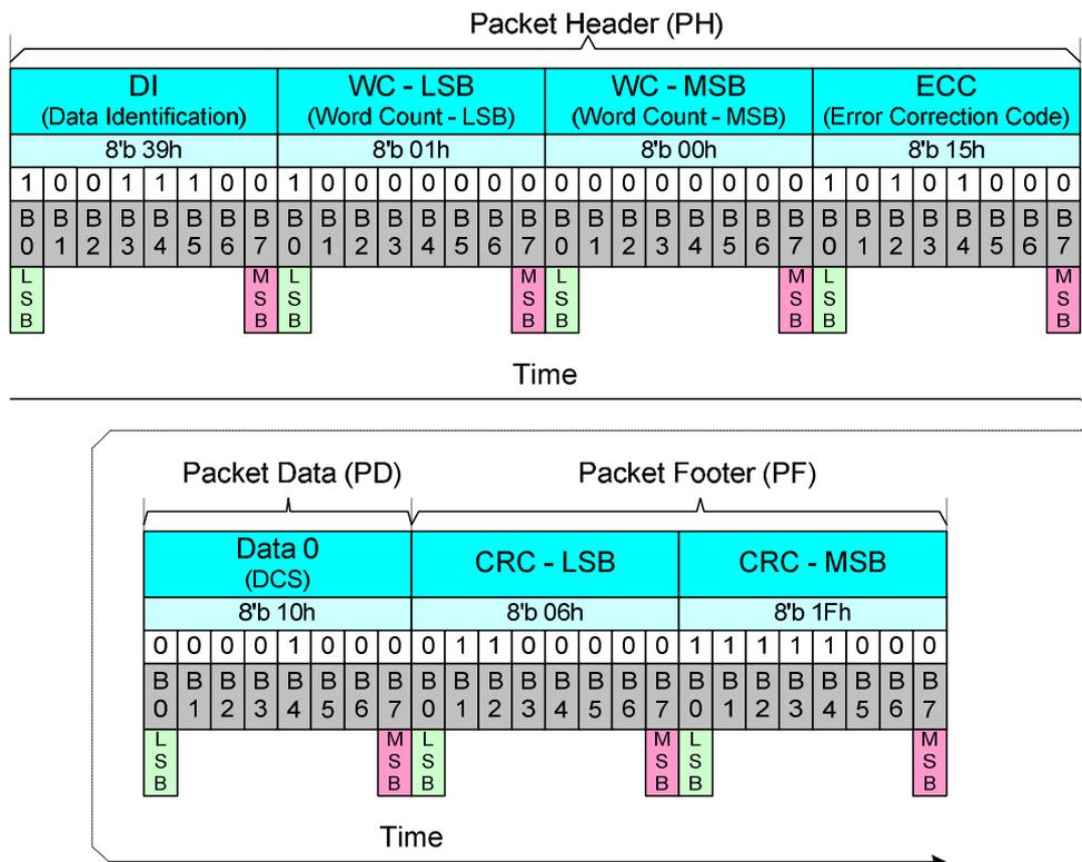
**Figure 68: Display Command Set Write Long (DCSW-L) with DCS Only – Example**
