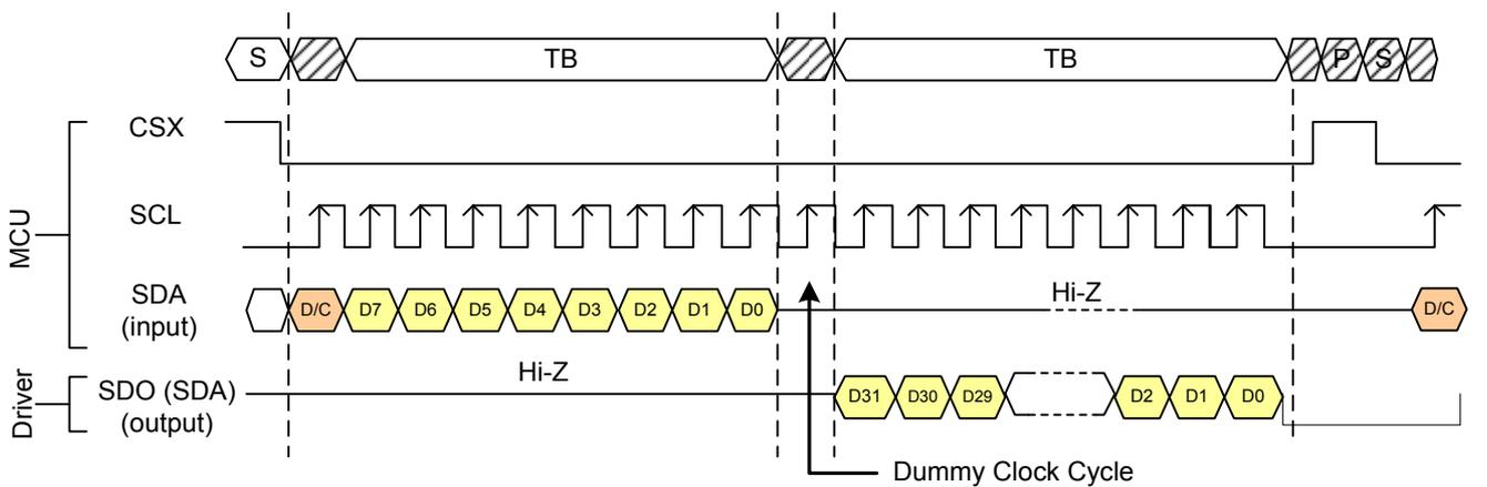
Figure 9: DBI Type C (Option 1) Read Cycle Sequence
