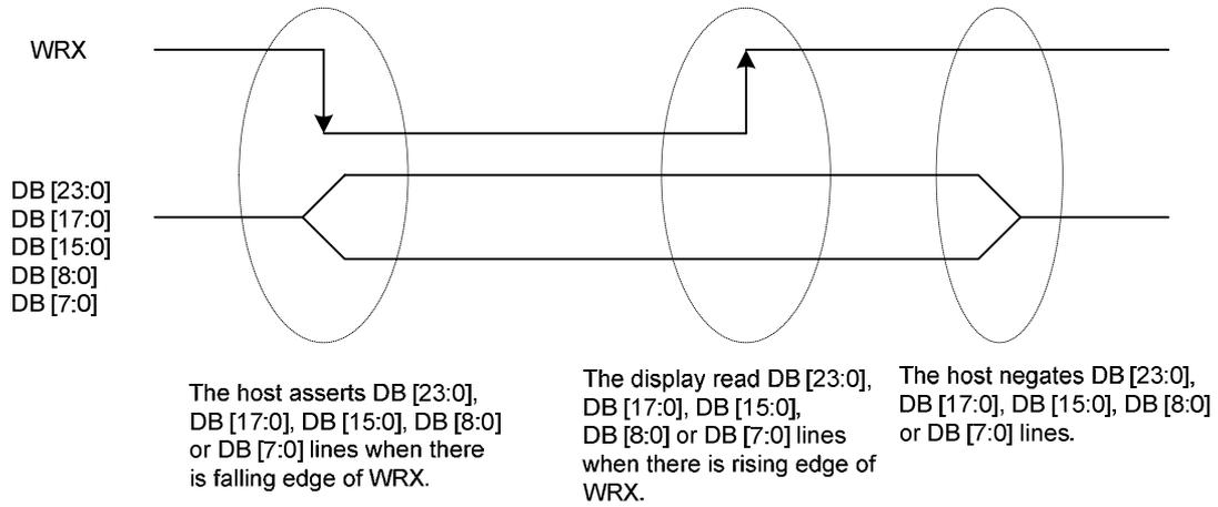
**Figure 1: DBI Type B Write Cycle**
