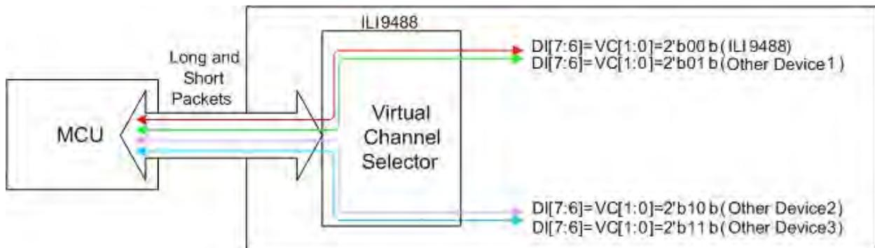
Virtual Channel (VC) is always 0 (DI [7..6] = VC [1..0] = 00b) when the MCU sends End of Transmission Packet to the display module.
