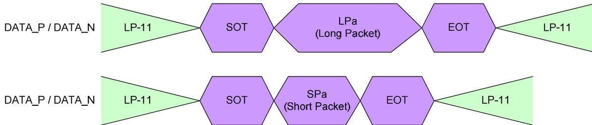
**Figure 39: Single Packet in High-Speed Data Transmission**
