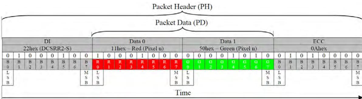
Figure 98: Red and Green Sub-pixels Response (DCSRR2-S) – Example 5
