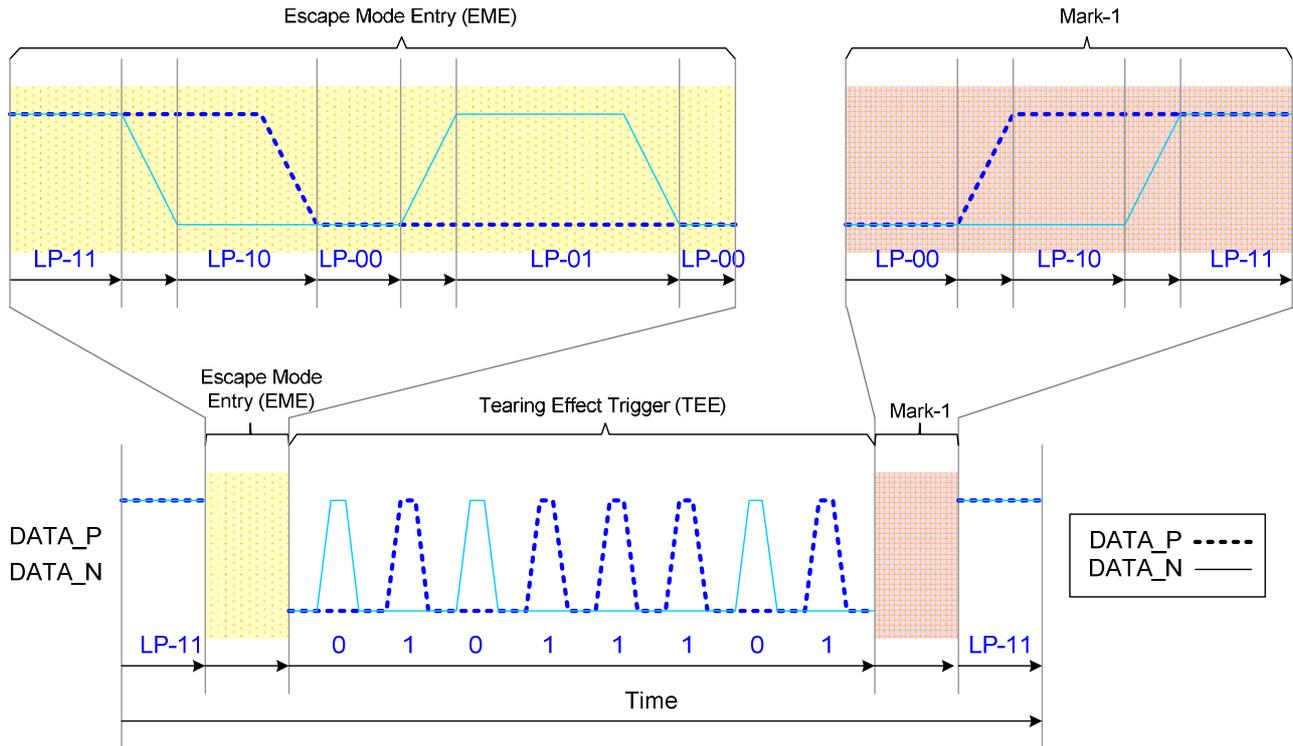
**Figure 35: Tearing Effect (TEE)**
