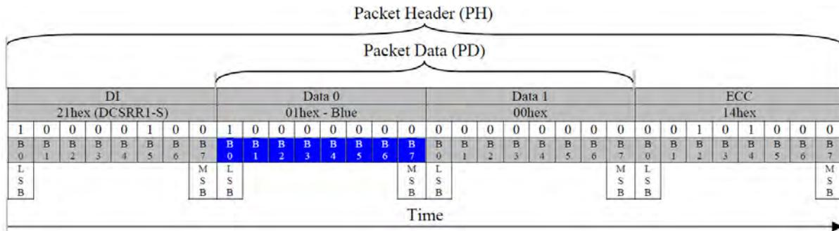
Figure 97: Blue Sub-pixel Response (DCSRR1-S) – Example 4
