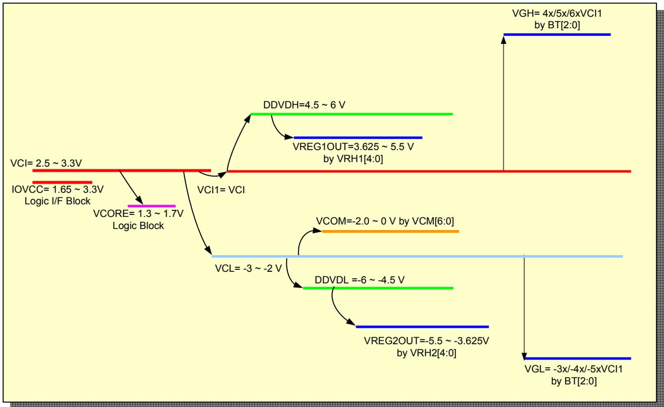
**Note:** The DDVDH, DDVDL, VREG1OUT, VREG2OUT, VCOM, VGH, VGL and VCL output voltage levels are lower than their theoretical levels (ideal voltage levels) due to the current consumption at respective outputs.
