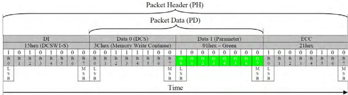
Figure 91: Green Sub-pixel Write (DCSW1-S) – Example 3
