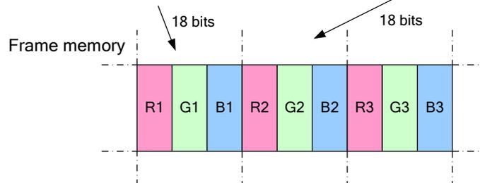
Note 1: The data order is as follows, MSB=D17, LSB=D0 and picture data is MSB=Bits 5, LSB=Bit 0 for Red, Green and Blue data.
