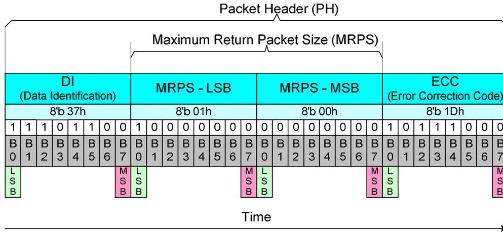
**Figure 71: Set Maximum Return Packet Size (SMRPS-S) – Example**
