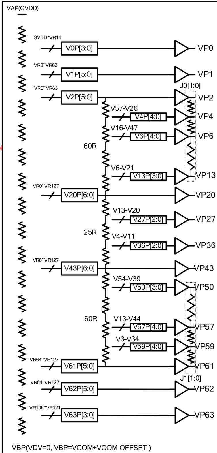
Figure 35 Gray scale Voltage Generation (Positive)
