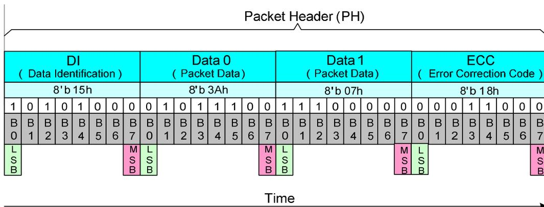
**Figure 46: Packet Header (PH) of Short Packet**
