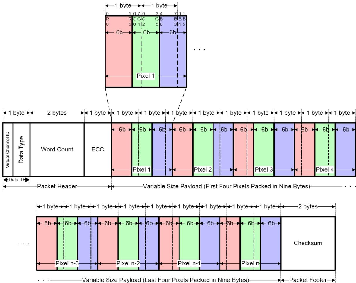
**Figure 126: 18-bit per Pixel, Data Type = 01 1110 (1Eh)**
