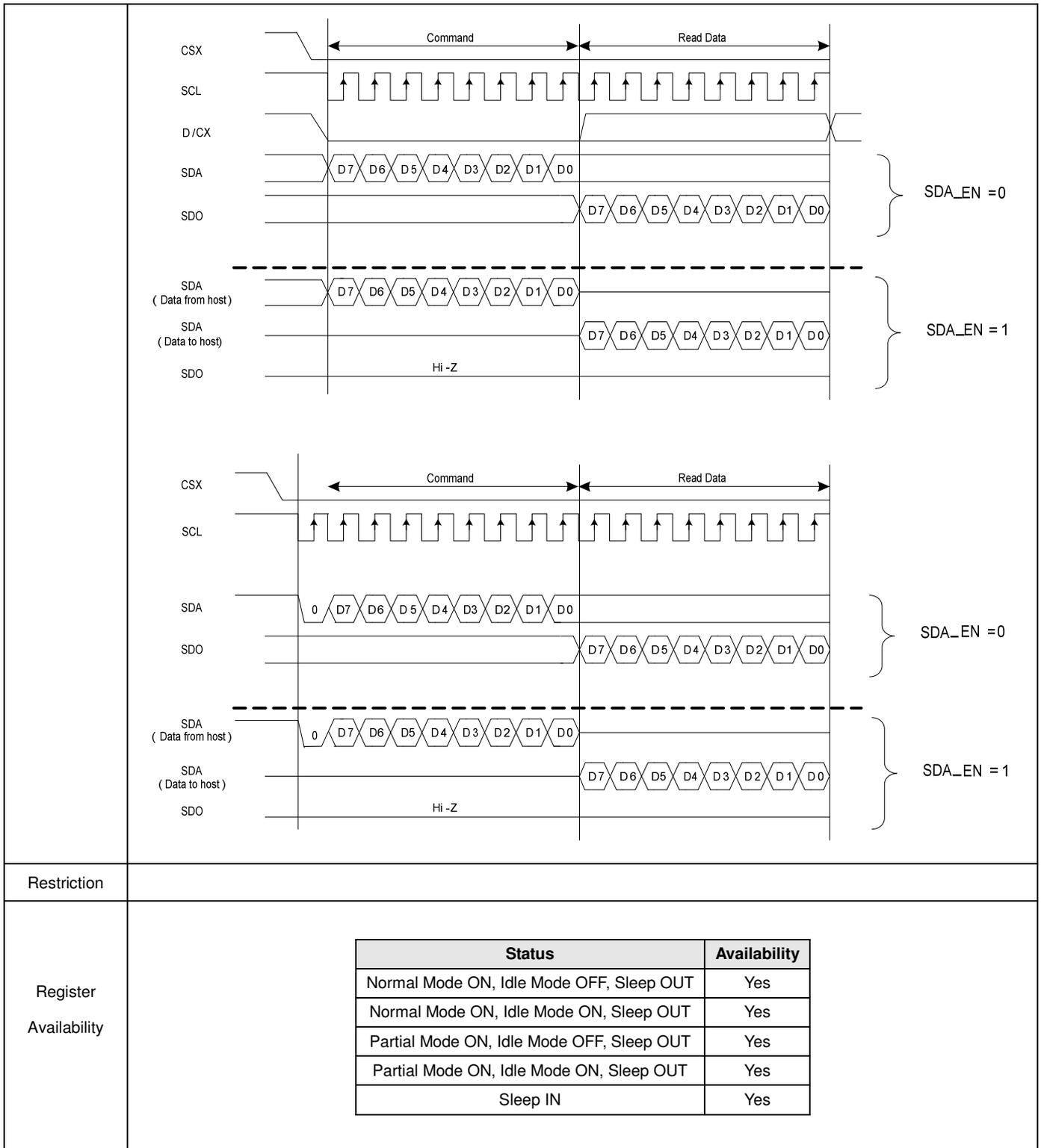
**5.3.2. Frame Rate Control (In Normal Mode/Full Colors) (B1h)**
