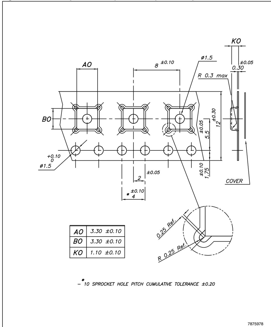
Figure 16. Reel information for QFN16 (3 x 3 x 1 mm) - 0.50 mm pitch
