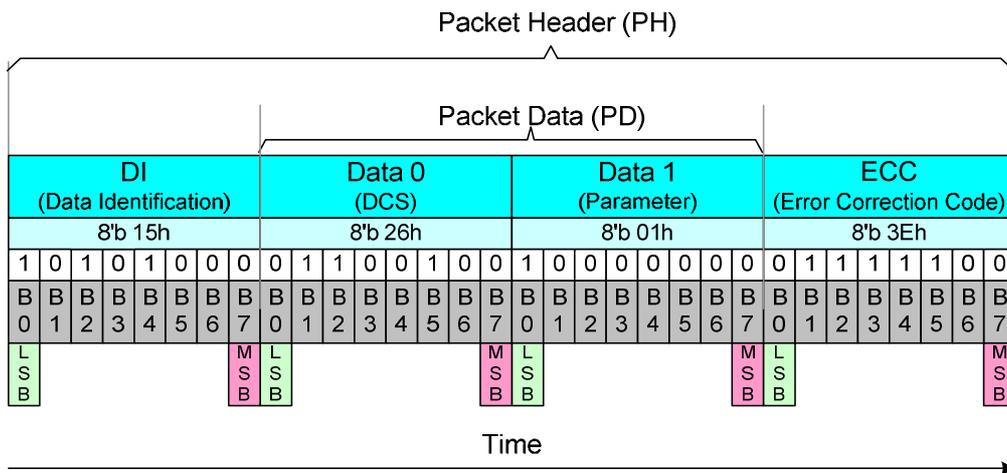
**Figure 67: Display Command Set Write, 1 Parameter (DCSW1-S) – Example**
