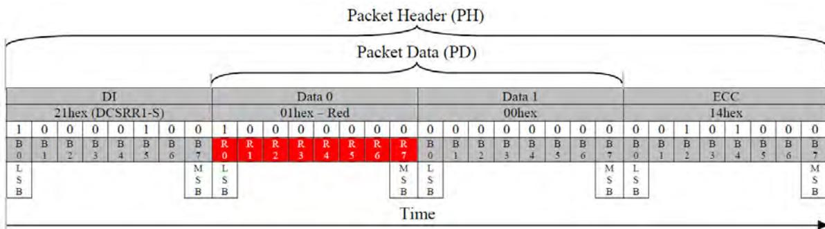
**Figure 95: Red Sub-pixel Response (DCSRR1-S) – Example 2**
