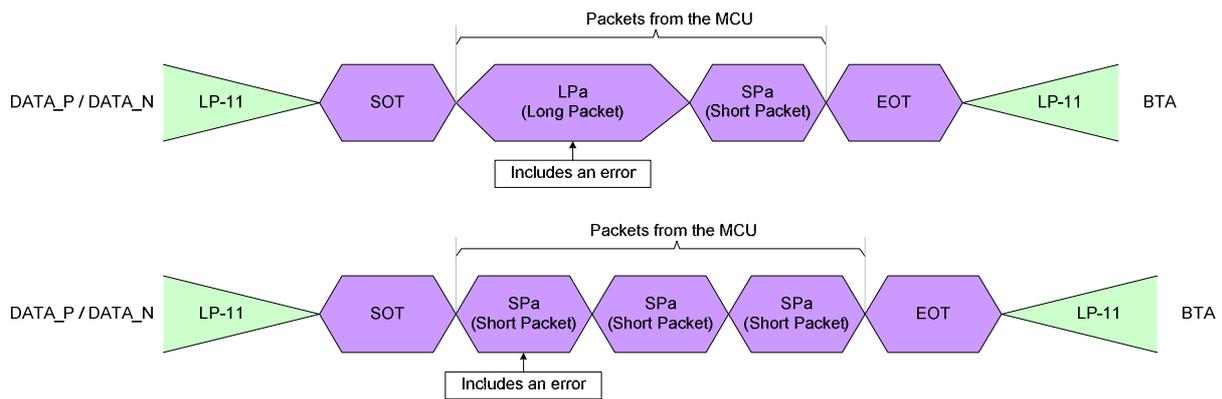
Therefore, a method is needed to check if there are errors in the previous packets. These errors of the previous packets are indicated by “Read Display Signal Mode (0Eh)” and “Read Number of the Errors on DSI (05h)” commands. If a received packet includes an error, the bit D0 of the “Read Display Signal Mode (0Eh)” command will be set to 1.
